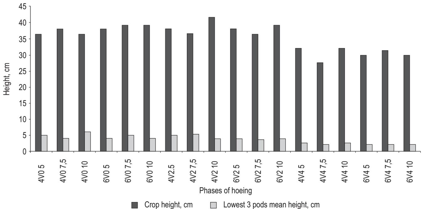
**Figure 2.** Crop height H and lowest three pod mean height h at phase "Physiological maturity" (R9), 2008–2010 year; 4V0.10 – hoeing in phase V0 at working speed of 10 km/h and working depth of 4 cm
