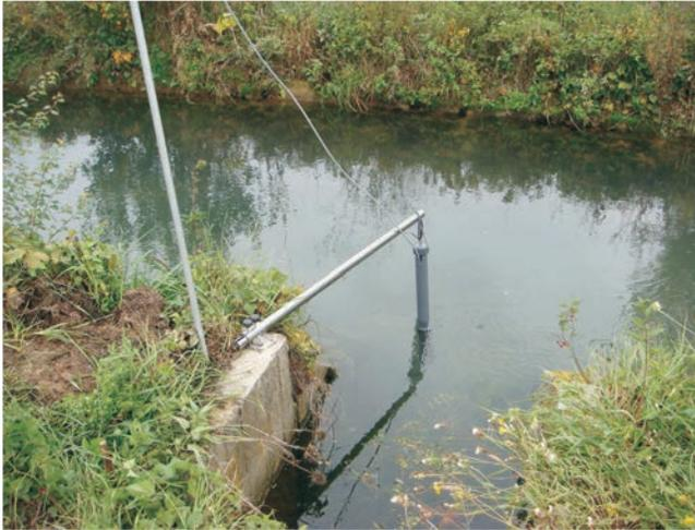
**Figure 1.** Mounting of the process probe for dissolved oxygen in the water supply channel
