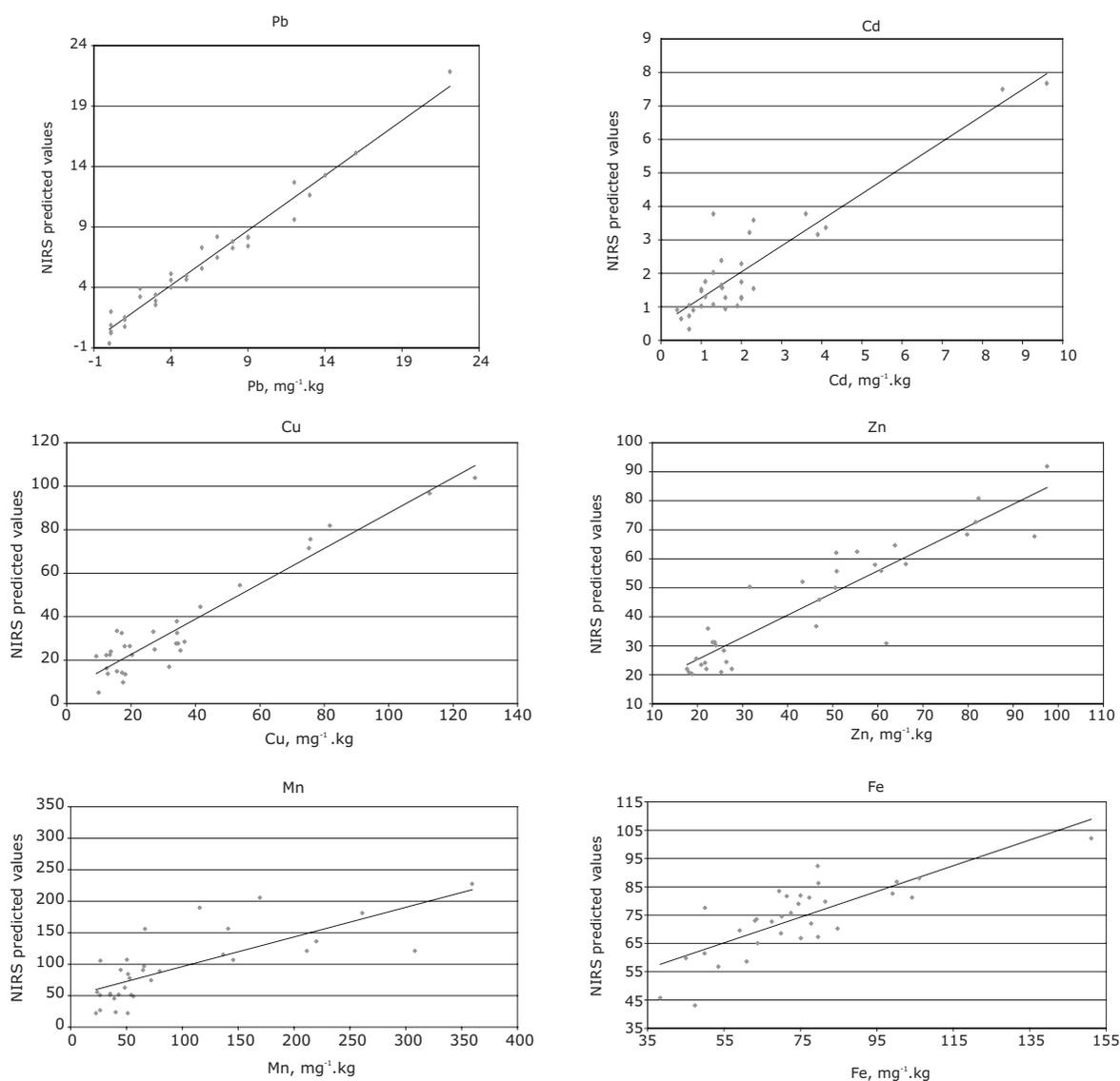
**Figure 1.** Comparison of reference values with the values predicted by the calibration equations for composition in trace elements (Pb, Cd, Cu, Fe, Mn and Zn) in tobacco.
