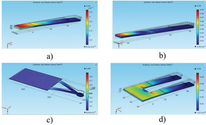
**Figure 2.** Stress induced in different cantilever designs subjected to a uniform loading: a) Simple cantilever; b) Sandwich cantilever; c) Triangular cantilever; d) C-beam cantilever
