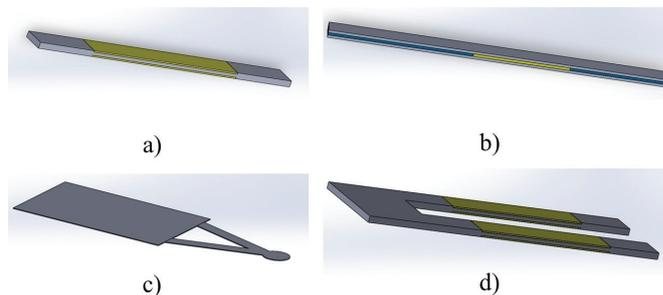
**Figure 1.** Different cantilever designs: a) Simple cantilever; b) Sandwich cantilever; c) Triangular cantilever; d) C-beam cantilever
