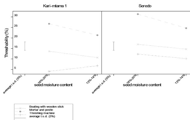
**Figure 4.** Mean percentage of mechanical damage for two sorghum varieties seeds threshed at two moisture content levels using three threshing methods (oven dried panicles)
