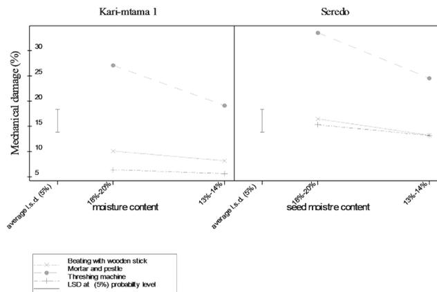
**Figure 3.** Mean percentage of mechanical damage for two sorghum varieties seeds threshed at two moisture content levels using three threshing methods (sun dried panicles)
