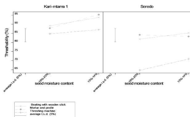
**Figure 1.** Mean percentage of threshability for sorghum panicles threshed at two moisture content levels using three threshing methods (oven dried panicles)
