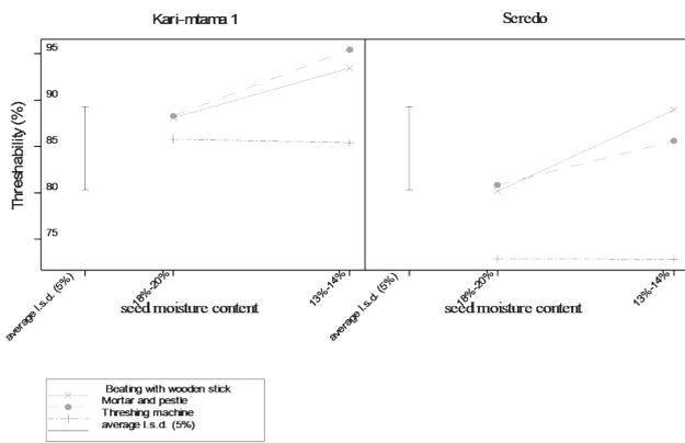
**Figure 2.** Mean percentage of threshability for sorghum panicles threshed at two moisture content levels using three threshing methods (sun dried panicles)
