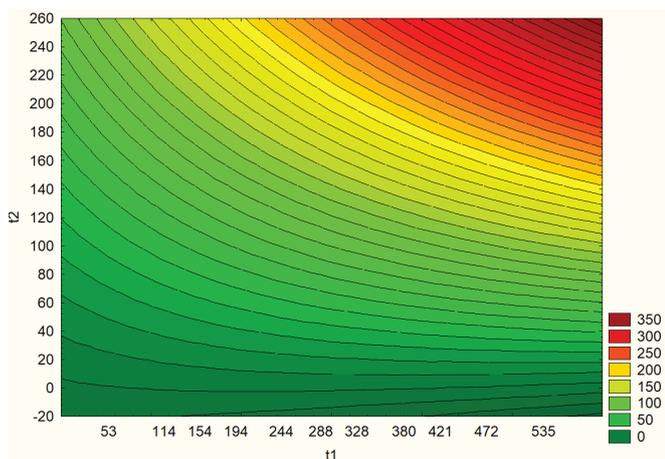
**Figure 2.** Lines of uniform response to the harvester idle time for unloading the hopper ( $T1$ ), depending on the time from activation of the alarm to the start of the vehicle ( $t_1$ ) and the time from the start of the vehicle to its arrival under the unloading auger of the grain harvester ( $t_2$ )
