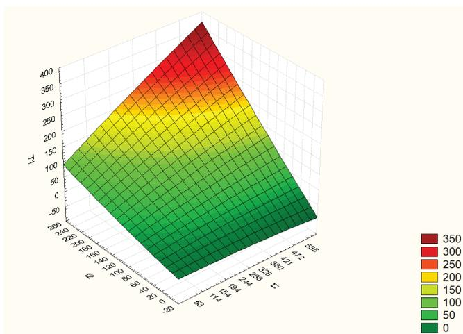
**Figure 1.** Change of harvester idle time for unloading the hopper ( $T1$ ), depending on the time from activating the alarm to the start of the vehicle ( $t_1$ ) and the time from the start of the vehicle to its arrival under the unloading auger of the grain harvester ( $t_2$ ) in different harvesters
